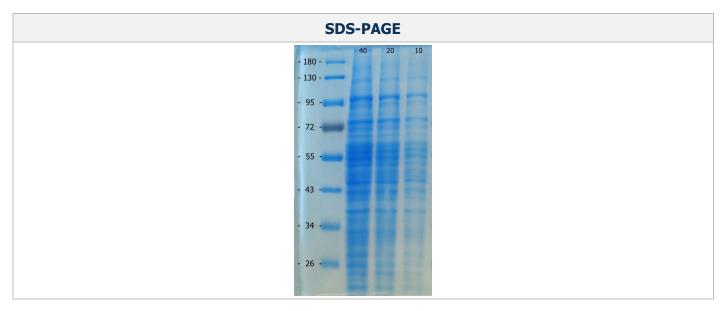
Note: SDS-PAGE was performed at PRIMACYT GmbH using a 7 % stacking gel and a 10 % separating gel with 10, 20 and 40 µg protein as indicated. Pageruler Prestained Protein Ladder by Thermo Scientific was used as marker. Protein sizes (kDa) denoted on the left.
